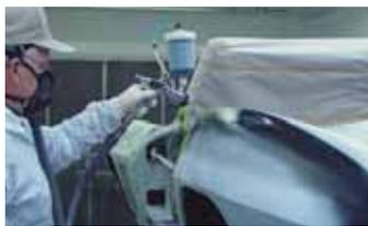
**High-Build Primer** - After spraying the epoxy primer, Darney applied a high-build primer to the body and all parts of the Vette. This primer was used to fill in minor imperfections, scratches, and low spots in the fiberglass. Also, the high-build primer saves time when block sanding because it goes on thicker and doesn't shrink like standard primer.
