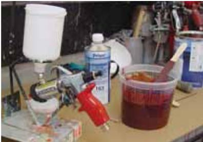
**Base Coat Mixing** - Darney used a Quick Mix Cup to mix the Milano Maroon base coat with their base coat stabilizer (#163) at a 1:1 ratio (1 part base coat to 1 part stabilizer). Darney said, "The Quick Mix Cups take the guess work out of mixing. They are inexpensive and have easy-to-read
