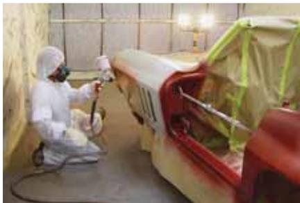
**Base Coat Application** - After the material was reduced, Darney strained the base coat and poured it into the paint gun. Next, he fired up the TP Turbine and started spraying the Vette body. Darney applied 4 coats of the Maroon to the Vette and loose body parts. He overlapped his spray pattern by 50% to avoid tiger striping and uneven metallic
