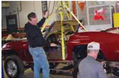
**Chassis Teardown** - Darney proceeded to strip the chassis down to the bare frame but ran into a bit of a letdown. After the rear end and drive shafts were removed, the rear section of the frame dropped to the ground! Years of moisture had weakened the metal just in front of the rear tires and caused severe rusting. After examining the rest of the frame, Darney decided to contact Vette Products in Michigan to order a new frame.
