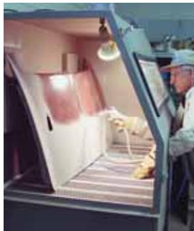
**Plastic Media Blasting - Body** - Darney also blasted the Vette body with the Skat Plus Plastic Abrasive and achieved the same fantastic results. Darney contacted Brut Mfg in Navarre, Ohio. Brut specializes in outdoor-type blasters for paint and rust removal - if it doesn't fit in the Skat Cabinet, give Brut a call at 1-888-533-2693.
