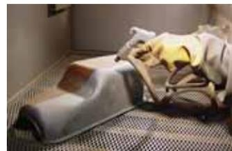
**Cabinet Blasting** - Before reassembling the motor and chassis, Darney blasted everything imaginable in the 1536 Skat Blast Cabinet -- engine pulleys, fan blade, oil pan, valve covers, brackets, a-arms, exhaust manifolds, drive shafts, control arms,
