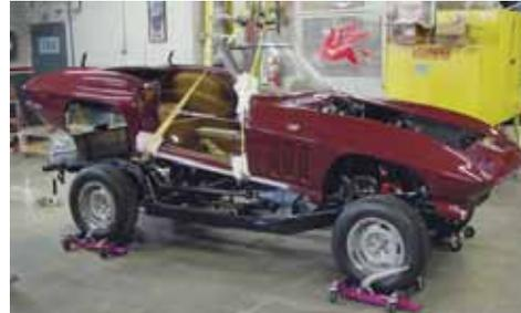
catalog shopping for all classic Corvette parts.) The body was then lowered to the frame with careful placement of shims between the
